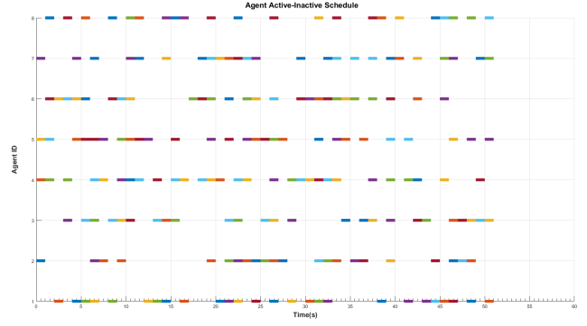
Figure 5: A Representative Figure of Schedule of Active/Inactive Agents for a time step of 1s. The colored lines represent that the agents are active for that time instant. A blank space for a time step represents that the agent is inactive for that time step.
